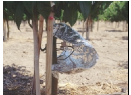
Linear variable displacement transducer used to measure trunk diameter fluctuations. Aluminum foil protects sensor from sun and wind.
