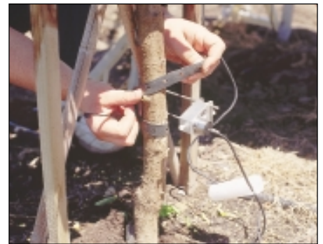
Attachment strap on mounting bracket of linear variable displacement transducer (LVDT) is affixed to the tree trunk.
