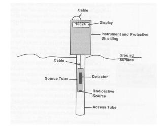
Fig. 1. Photo and schematic of a neutron probe.
